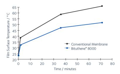
Comparsion of solar heat gain over time on exposed membrane samples.
